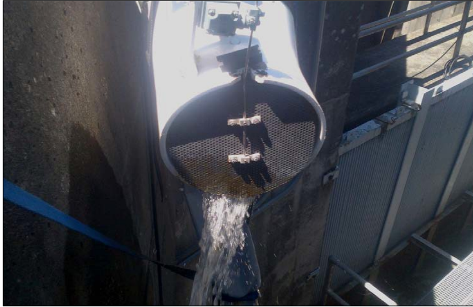
Figure 19. Exit chute counting mechanism on BON Washington Shore AWS Channel LPS. Lamprey exiting the system actuate the perforate plate paddle, which is connected to a digital counter. Counting systems are still in development.
